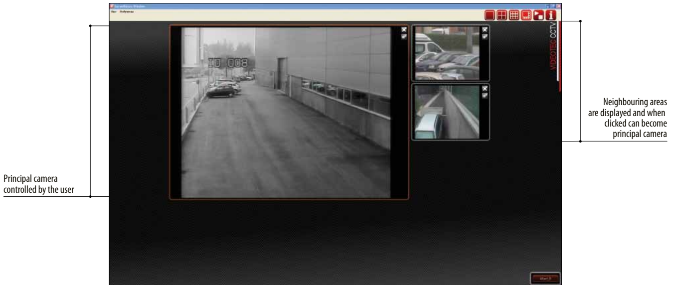
EXAMPLE OF ASSISTED NAVIGATION AT VIDEOTECH'S INSTALLATION
