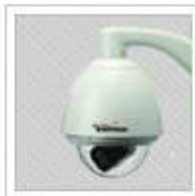
Speed Dome Camera
