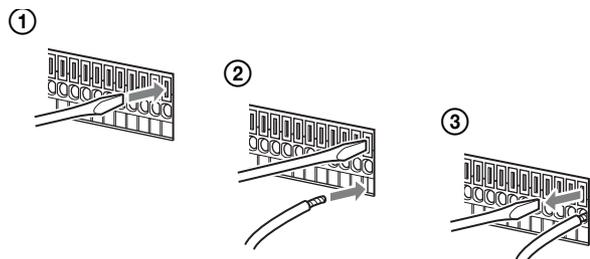
Repeat this procedure to connect all required wires.
