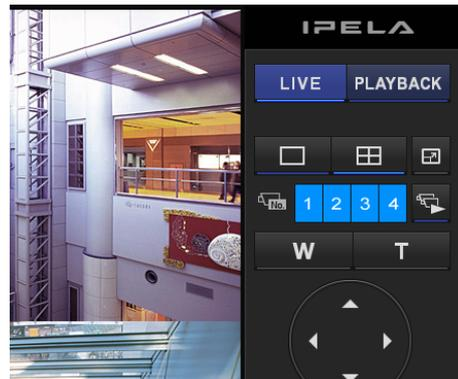
You can set the display time for each monitor frame. For details on how to make this setting, refer to “AutoScan Period” (page 39) in “System Setting” Screen Details”.
