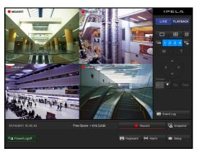
Continuous recording starts automatically after the cameras are registered.
