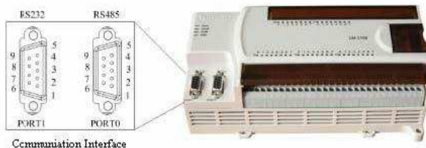
Figure 2-7-4 LM3108 Communication Interface
