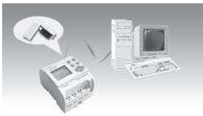
Fig. 4 . 24. FAB Communication Connection Frame
